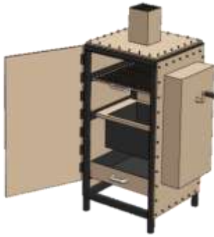
Fig. 1. Charcoal fired fish smoking kiln
